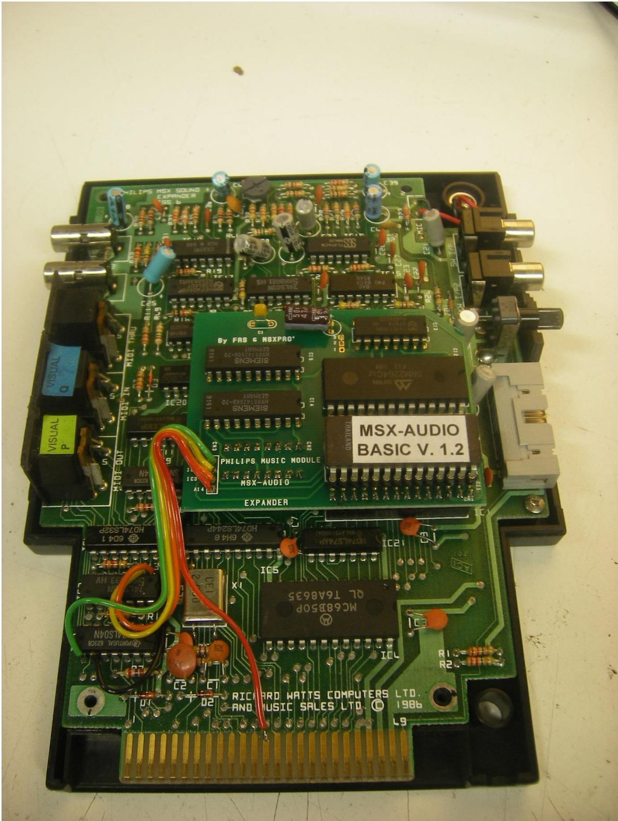
Philips NMS 1205 Music Module with installed expansion board.
