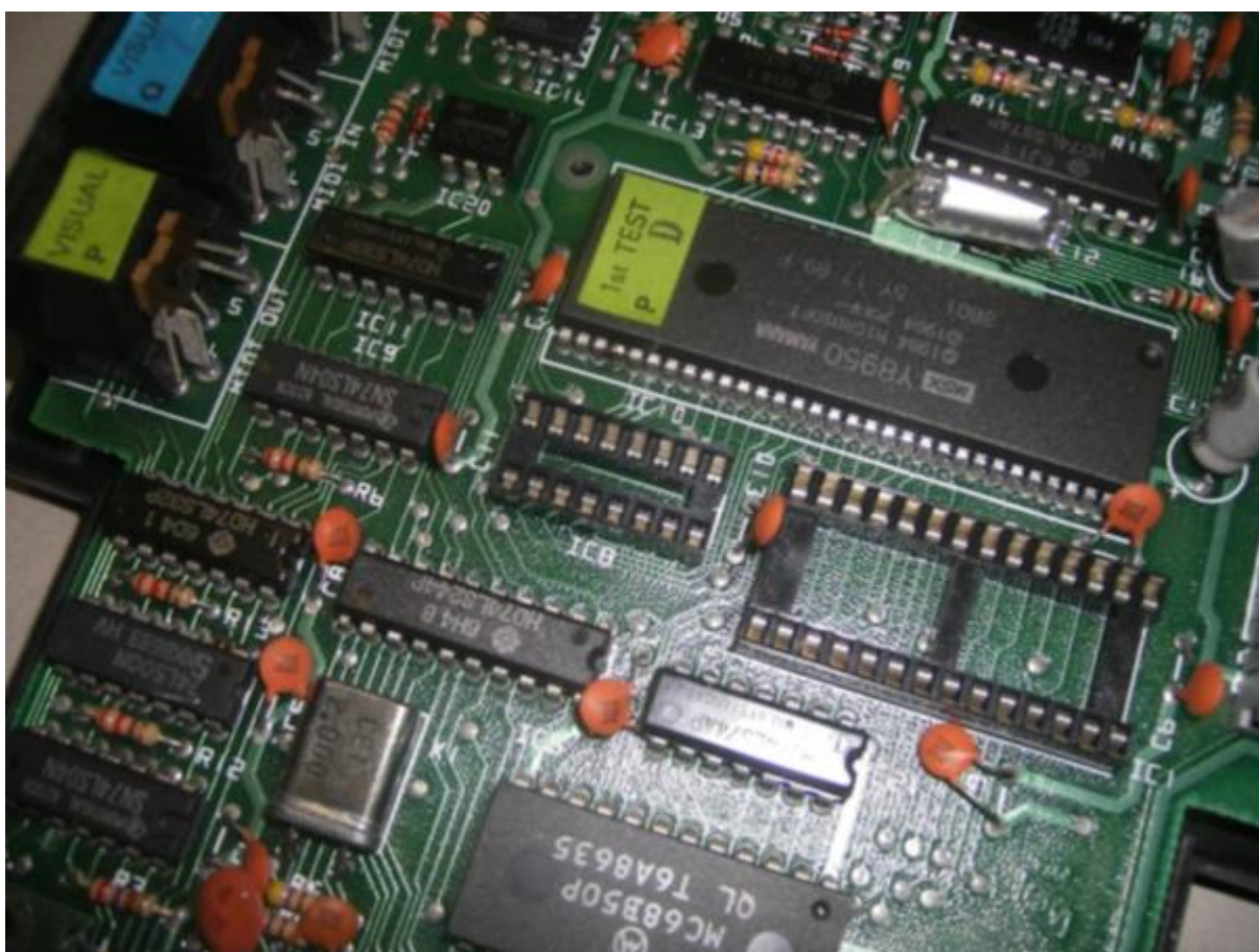
IC1 has been removed and IC8 has been replaced by an IC socket.
